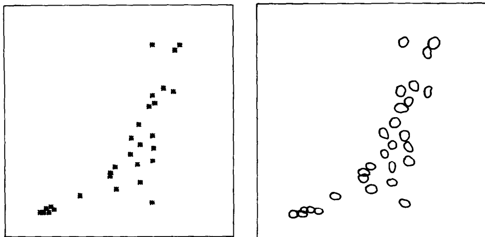
Fig. 6. Computer-simulated (left) and experimental (right) chromatograms for two-dimensional chromatography performed on a silica gel plate. The vertical axis is a butyl acetate-toluene development (mole fraction 0.1, development time 1430 sec), the horizontal axis is a tetrahydrofuran-toluene development (mole fraction 0.2, development time 860 sec). The solvent path length in each dimension is 8.3 cm. The above diagrams are for a 10 \times 10 cm plate which includes the solvent evaporation area.
